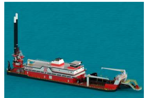
WEEKS MARINE J.S. Chatry 2 x 16V250MDC and 3 x 8L250MDC (Mechanical Pump Drive and Diesel Electric Power) Cutter Head Dredging Vessel
