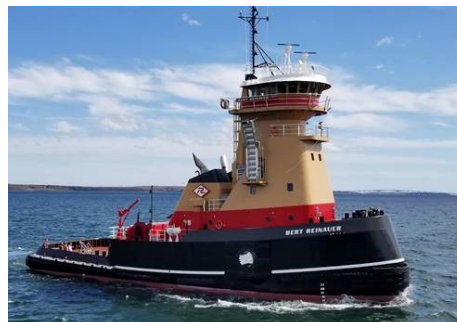
REINAUER TRANSPORTATION M.V. Bert Reinauer 2 x 12V250MDC (Mechanical Propulsion) Articulated Tug Barge (ATB)
