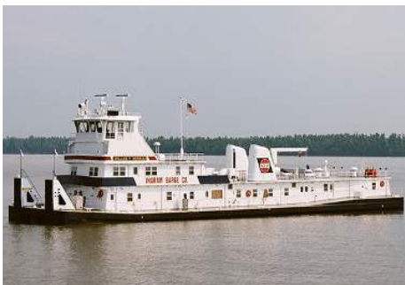
INGRAM BARGE COMPANY M.V. Mark Duley 2 x 8L250MDC (Mechanical Propulsion) Inland Marine Tow Boat
