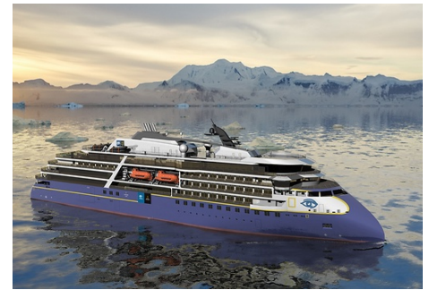
LINDBLAD EXPEDITIONS M.V. National Geographic Endurance 2 x 8L250MDC and 2 x 12V250MDC (Diesel Electric Power and Propulsion) Arctic Excursion Cruise Vessel
