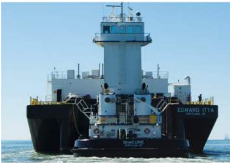
HARLEY MARINE M.V. Harley One Cure 2 x 6L250MDC (Mechanical Propulsion) Articulated Tug Barge (ATB)
