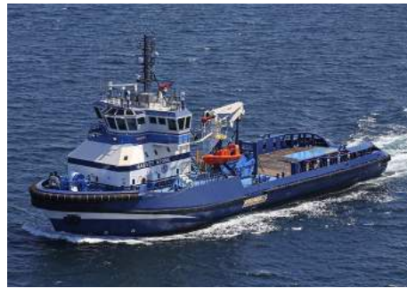
HARVEY GULF M.V. Harvey Stone 2 x 12V250MDC (Diesel Electric Power and Propulsion) Multi-Purpose Field Support Vessel (MPFSV)
